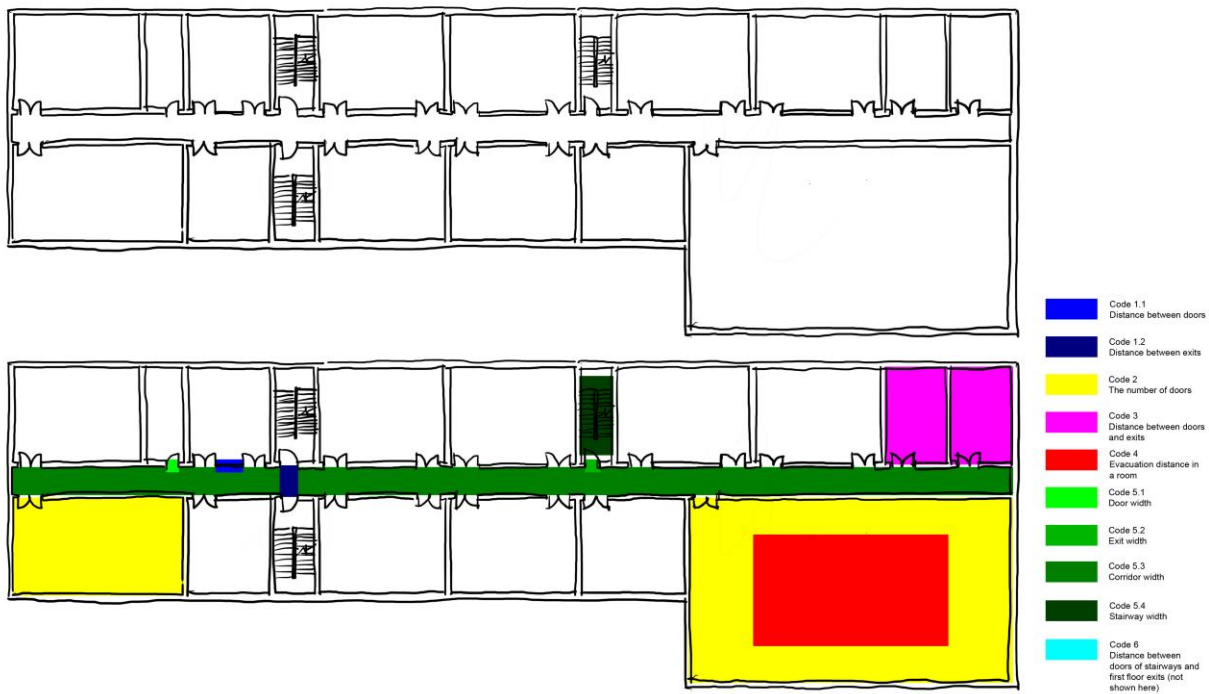
Figure 3: Input image and checked image with color marks for nine checking functions.
