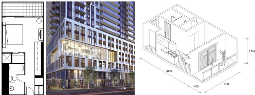
Figure 2: Plan, section and exterior photograph of the Dundas Square Gardens, Unit type G24, designed in 2019, unit aspect ratio 1:1.8.
